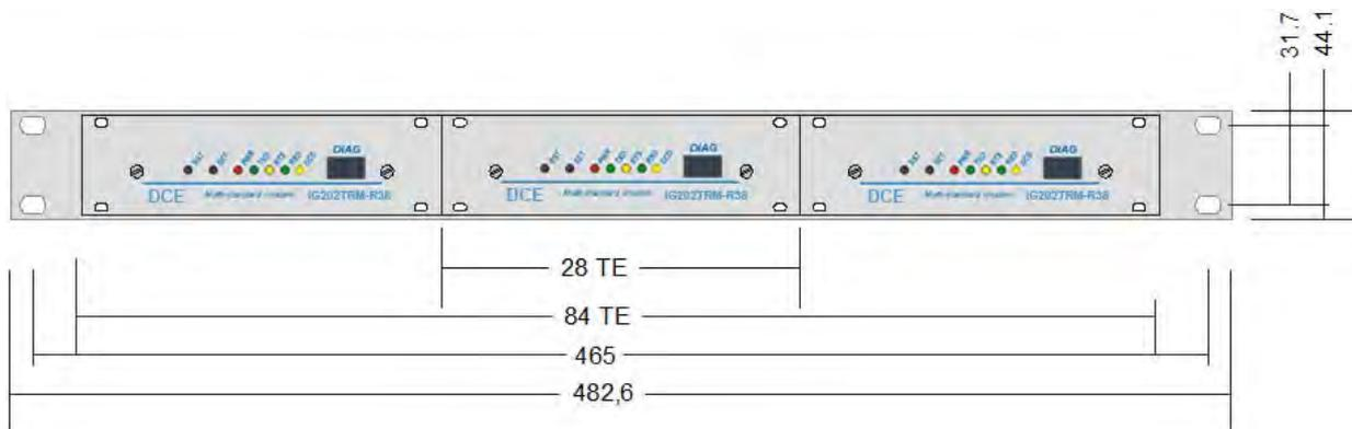
Figure A1b. Rack frame 1U/84TE - Rear view
