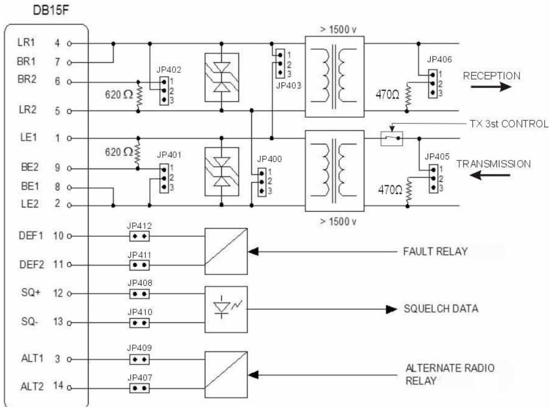
Figure 4. Analog line interface
