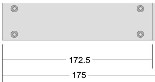
Figure A1d. Rack 1U/28TE - Front plate view
