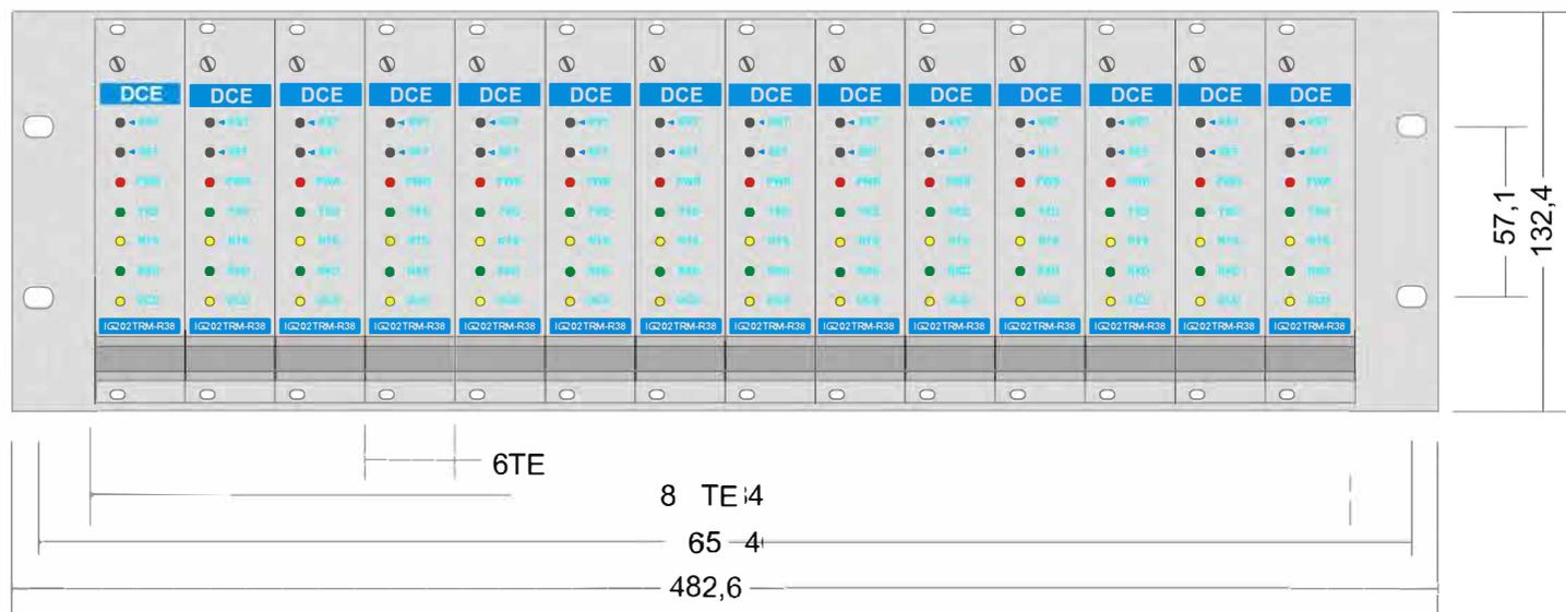
Figure A2b. Rack frame 3U/84TE - Rear view
