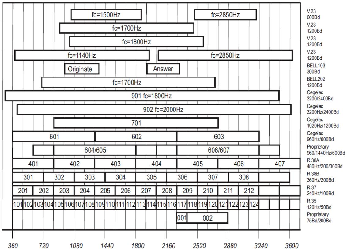
Figure 1. Table of programmable channels in FSK mode
